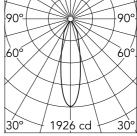
Luminous flux luminaire 594 lm (EXTREME CUT OFF)
