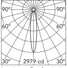
Luminous flux luminaire 684 lm (EXTREME CUT OFF)
