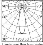
Luminous flux luminaire 722 lm (EXTREME CUT OFF)
