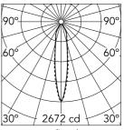
Luminous flux luminaire 715 lm (EXTREME CUT OFF)
