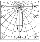
Luminous flux luminaire 752 lm (EXTREME CUT OFF)
