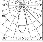
Luminous flux luminaire 396 lm
