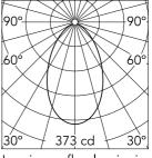
Luminous flux luminaire 910 lm
