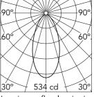
Luminous flux luminaire 950 lm
