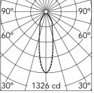
Luminous flux luminaire 591 lm (EXTREME CUT OFF)
