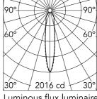
Luminous flux luminaire 601 lm (EXTREME CUT OFF)
