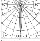
Luminous flux luminaire 357 lm
