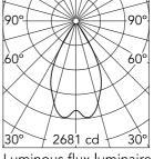
Luminous flux luminaire 2367 lm
