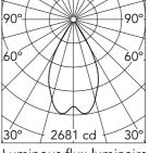
Luminous flux luminaire 2367 lm
