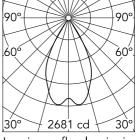
Luminous flux luminaire 2367 lm
