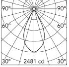
Luminous flux luminaire 1371 lm
