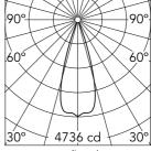
Luminous flux luminaire 1403 lm
