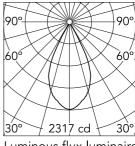
Luminous flux luminaire 1280 lm
