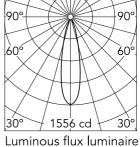
24° Beam Angle: h(m) = E(Ix)D(m) 1556 0.43 2 389 0.85 3 173 1.28 4 97 1.71 5 62 2.14
