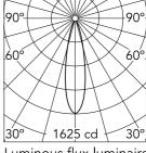
Luminous flux luminaire 340 lm
