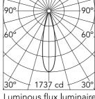
24° Beam Angle: h(m) = E(Ix)D(m) 1737 0.42 2 0.84 434 3 193 1.26 4 109 1.68 5 69 2.10
