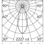
Luminous flux luminaire 1085 lm
