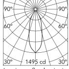
Luminous flux luminaire 655 lm
