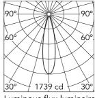
Beam Angle: 23° h(m) = E(Ix)D(m) 1739 0.41 2 0.83 435 3 193 1.24 4 109 1.66 5 70 2.07
