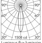
30° 1508 cd 30° 5 60 Luminous flux luminaire 240 lm
